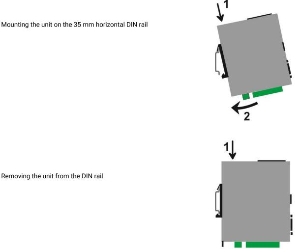
Mounting the unit on the 35 mm horizontal DIN rail
