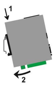
Removing the unit from the DIN rail
