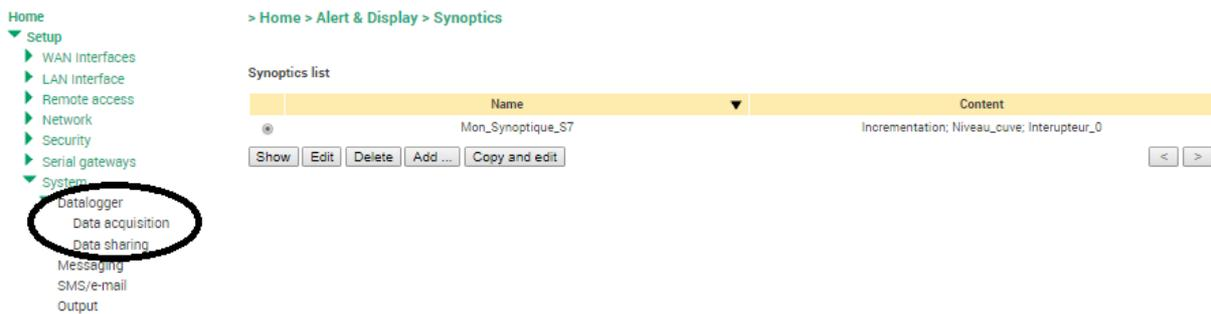
Click "Data Acquisition" to create an archive file. You can then define the variables to be archived, the recording period, the column separator (; in the example below) and the maximum file size.
