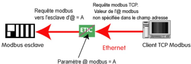
**Warning :** Several TCP Modbus client can send requests to the slaves on the serial link. Nevertheless, care must be taken not to saturate the serial link since its flow rate is much lower than the Ethernet one.
