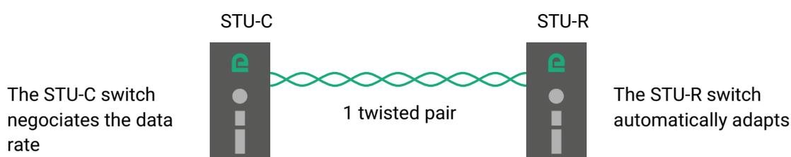
**One switch is normally configured as a STU-C and the other as a STU-R. However, to make the configuration simpler, the switch configured as a STU-C is able to automatically change to STU-R mode if it detects the presence of a STU-C on the remote side. Thus, two XS configured both in STU-C will find a way to connect. One of the two will switch to STU-R.**
