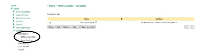
Click "Data Acquisition" to create an archive file. You can then define the variables to be archived, the recording period, the column separator (; in the example below) and the maximum file size. NB: to create the file, do not forget to click on "Enable" and "Save".
