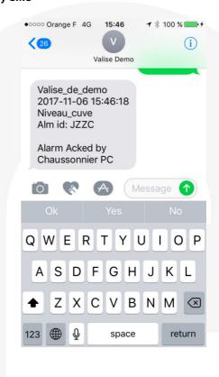
The alert can also be acknowledged locally when the Etic Telecom product has a digital input (dry contact). The digital input is available on all RAS / IPLs except the RAS-E-100, IPL-E-100, RAS-C-100, IPL-C-100, RAS-EW-100, IPL-EW -100. You can also acknowledge an alarm from the operating menu of the Etic Telecom box (see chapter 9).
