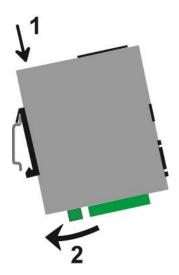
Removing the unit from the DIN rail
