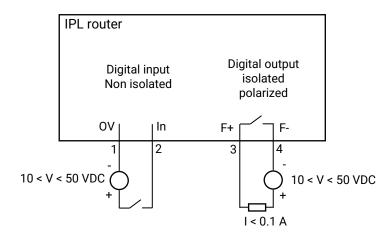
To check that the input and the output are correctly wired :
