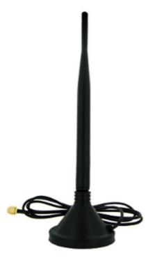
The mobile antenna is designed for installation on a vehicle or on a metal surface. The magnetic attachment system is easy to be removed as the solution does not require drilling, the cable being positioned on the side. It comes with a 1m cable with a RP-SMA-connector plug.
